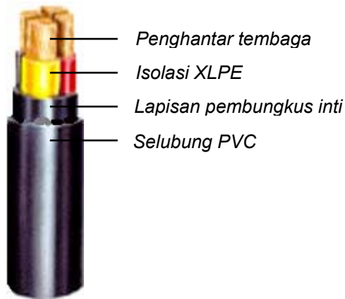
Gambar 2.30 Kabel N2XY
